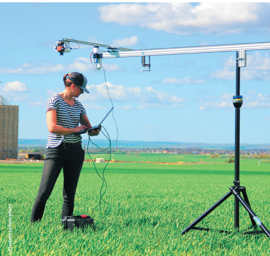
Above: Marja Haagsma operates a mobile, tripod-mounted HyperRail above a wheat field in Pendleton.
